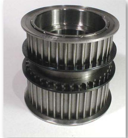
**Customer Situation:** MarquipWardUnited, a manufacturer of finishing equipment for the corrugated machinery was bolting two idler pulleys of different widths and diameters together in an effort to run two drive belts within close proximity of each other. The bolted pulleys were unable to maintain concentricity and were a costly attempt at solving the problem.
