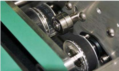
**Customer Situation:** GBR Systems Corp., a manufacturer of paper handling equipment, was using set screws to connect a high-speed drive pulley, running a Gates Polyflex JB belt, to a 3/8 in. shaft. The set screws would loosen during clutching and breaking at high RPMs, causing the machine to malfunction and damage to the belt. Constantly tightening the set screws resulted in loss of machine productivity and increased maintenance costs.
