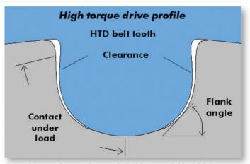
Second generation synchronous belt drives are dubbed 'high torque drive' and use a curvilinear profile for the belt and sprocket teeth.
