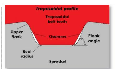
First generation synchronous belts featured trapezoidal tooth forms and delivered positive drive and greater efficiency than v-belt drives. Under load, the teeth mesh with the mating pulley teeth at the pulley's tooth root radius and the upper flank of the pulley tooth on the tight side of the belt.
