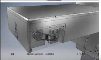
Hine's forward-thinking philosophy lets their engineers proactively seek out new and innovative (as well as cost-effective) ways to improve their products and enhance customer-service flexibility. Shown here is a detail of the axis inside the SL-2000 that uses the Concentric Maxi Torque assemblies.
